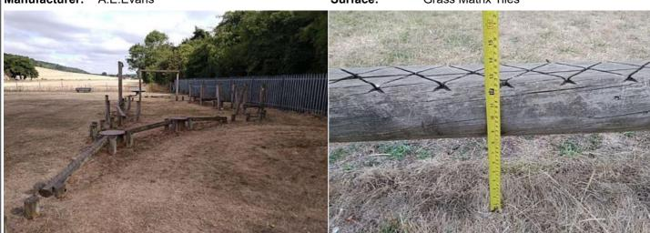
**Finding:** The clearance to the underside of the beam is less **Action:** Monitor - no remedial action recommended than 400mm and fails the requirements of BS EN 1176 Part
