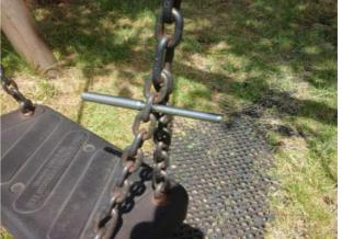
**Finding:** The chain openings are in excess of the 8.6mm as recommended by BS EN 1176
