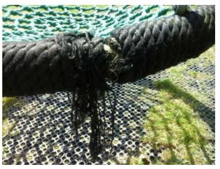
Finding: The seat is severely damaged and requires replacing
