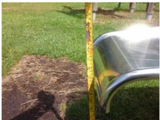
The height of the slide runout is in excess of 350mm and fails the requirements of BS EN Finding:
