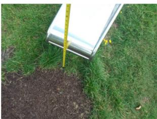
The height of the slide runout is in excess of 350mm and fails the requirements of BS EN Finding:
